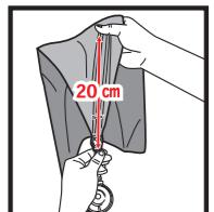
When injecting gas with the precision inflator (low-pressure injection device), pull upwards while holding them approximately 20 cm away from the inlet (film valve) as shown in the figure.
